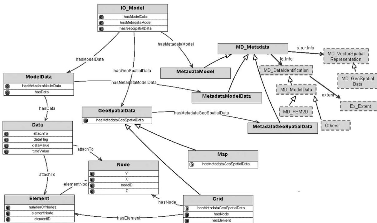
Figure 1 | Data and metadata ontology for hydrodynamic codes.
