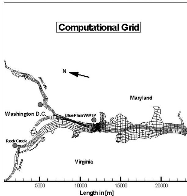
Figure 3 | Numerical grid of the Upper Potomac River.
