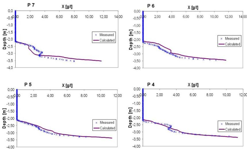
Figure 3 | Comparison of measured and calculated SS concentrations in representative vertical profiles of the SST.
