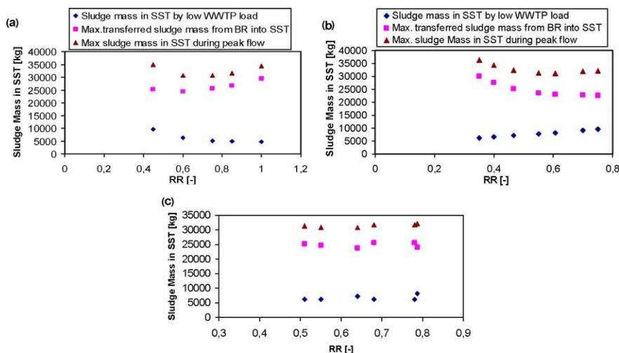
**Figure 7** | Sludge mass in the SST at peak flow event. (a) Adaptation of the return sludge flow to the current load of the WWTP with a constant recycling ratio ( $RR = Q_{RS}/Q = \text{const.}$ ); (b) Constant return sludge flow rate independent from the current load of the WWTP ( $Q_{RS} = \text{const.}$ ); (c) Increasing the return sludge flow in a way proportional to the increase of the WWTP load, applied above a threshold inflow, and shifted in time.
