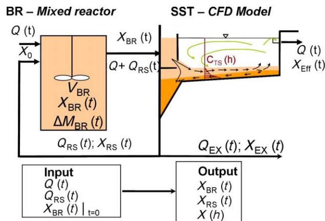
**Figure 1** | Scheme of the mass transport model.
