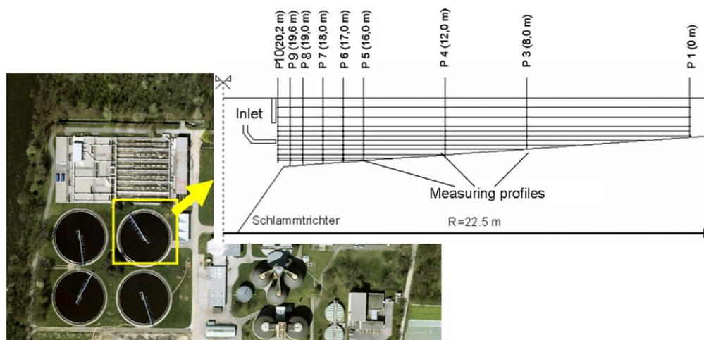
**Figure 2** | Top view of the secondary settling tanks in the WWTP of Graz with displaying the geometry and measuring raster of the investigated tank.
