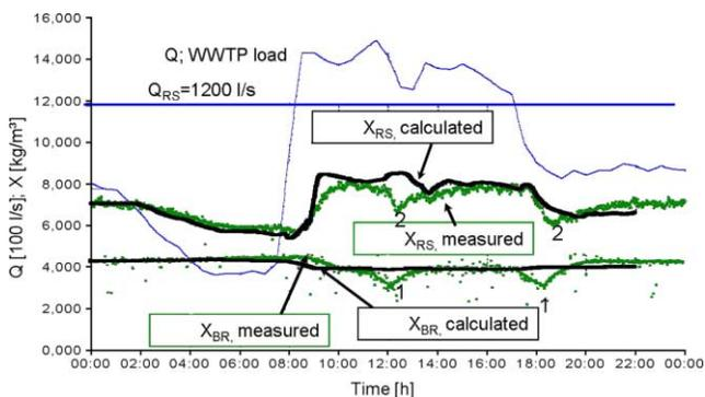
Figure 4 | Comparison of measured and calculated concentrations of return sludge and SS in the BR.
