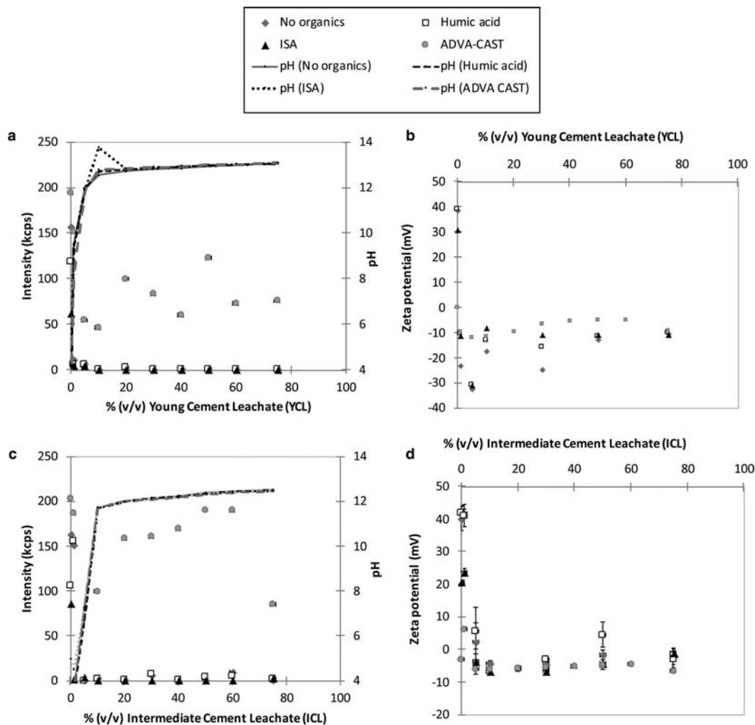
Fig. 6. Light scattering intensity and Zeta potential as a function of the percentage of cement leachate for  $\text{Fe}_2\text{O}_3$  colloids in the presence of YCL (a) light scattering and (b) Zeta potential and in the presence of ICL (c) light scattering and (d) Zeta potential.
