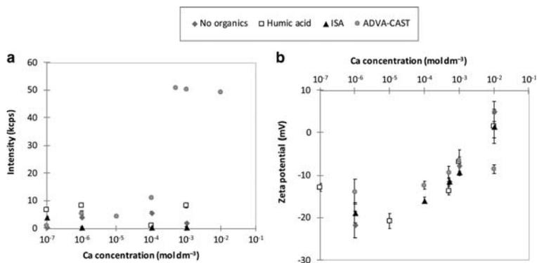
Fig. 4. Stability of Fe<sub>2</sub>O<sub>3</sub> colloids as a function of the concentrations of Ca (as Ca(NO<sub>3</sub>)<sub>2</sub>) (a) light scattering and (b) Zeta potential.
