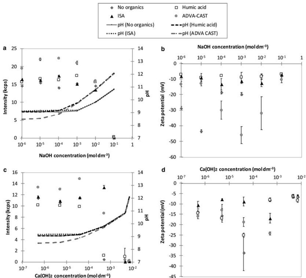
Fig. 2. Light scattering intensity and Zeta potential as a function of the pH for silica colloids in the presence of NaOH (a) light scattering and (b) Zeta potential and in the presence of Ca(OH)<sub>2</sub> (c) light scattering and (d) Zeta potential.
