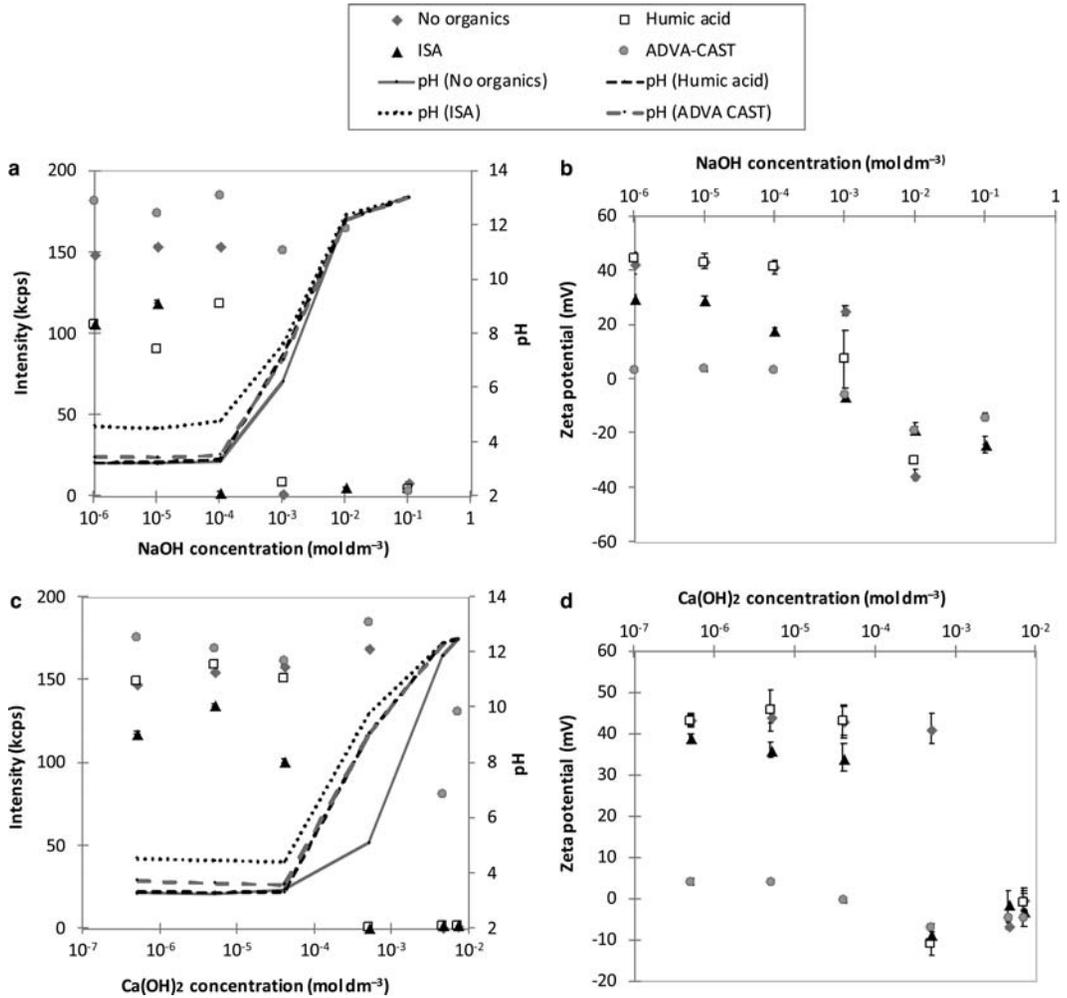
FIG. 3. Light scattering intensity and Zeta potential as a function of the pH for  $\text{Fe}_2\text{O}_3$  colloids in the presence of NaOH (a) light scattering and (b) Zeta potential and in the presence of  $\text{Ca}(\text{OH})_2$  (c) light scattering and (d) Zeta potential.
