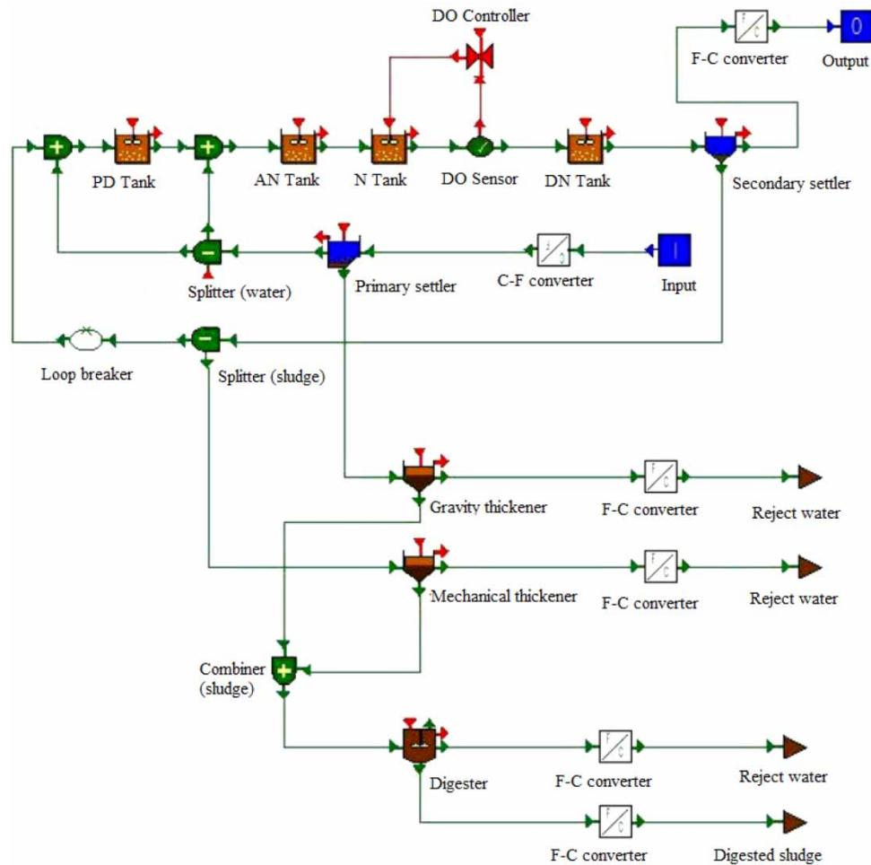
**Figure 1** | Setup of the plant model in WEST<sup>®</sup> 3.7.6.
