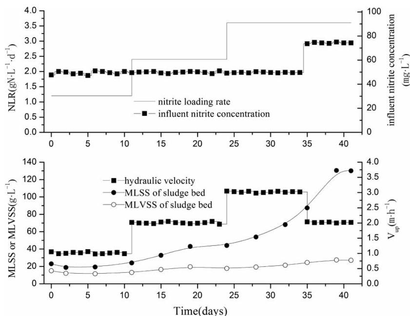
Figure 2 | Nitrite loading operation and biomass concentration of the reactor in the cultivation of nitrite granular sludge.
