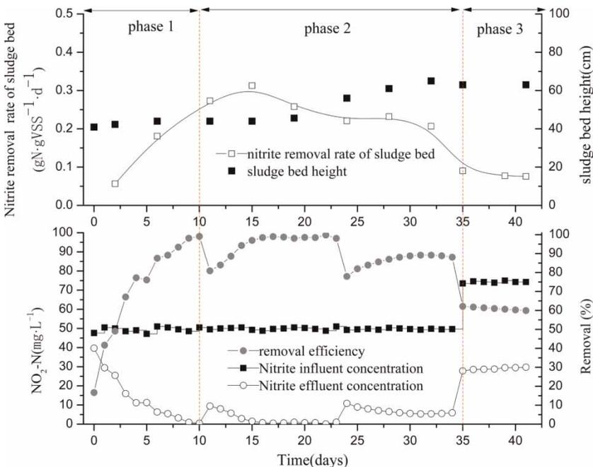
Figure 3 | Nitrite removal rate of nitrite granular sludge in the USB reactor.
