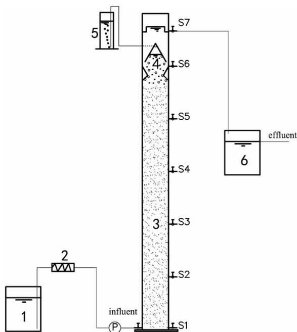
**Figure 1** | A schematic diagram of experimental equipment. 1: feed tank; 2: thermostatic bath; 3: USB reactor; 4: three phase separator; 5: water seal; 6: effluent tank; P: metering pump.
