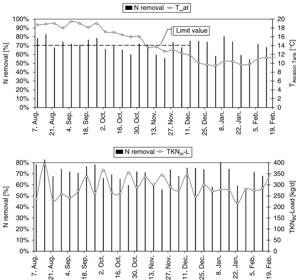
Figure 5 | WWTP Knittelfeld: total nitrogen removal, aeration tank temperature (upper figure) and TKN-influent load (lower figure) for the period Aug 2006–Feb 2007.
