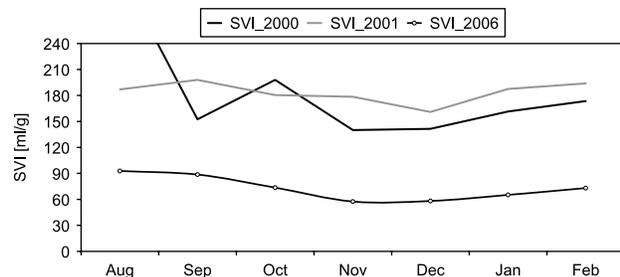
Figure 6 | WWTP Knittelfeld: sludge volume index before (2000/2001) and after (2006) extension of the plant.
