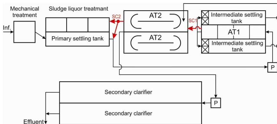
Figure 4 | Layout of WWTP Knittelfeld after plant extension according to the HYBRID®-concept.
