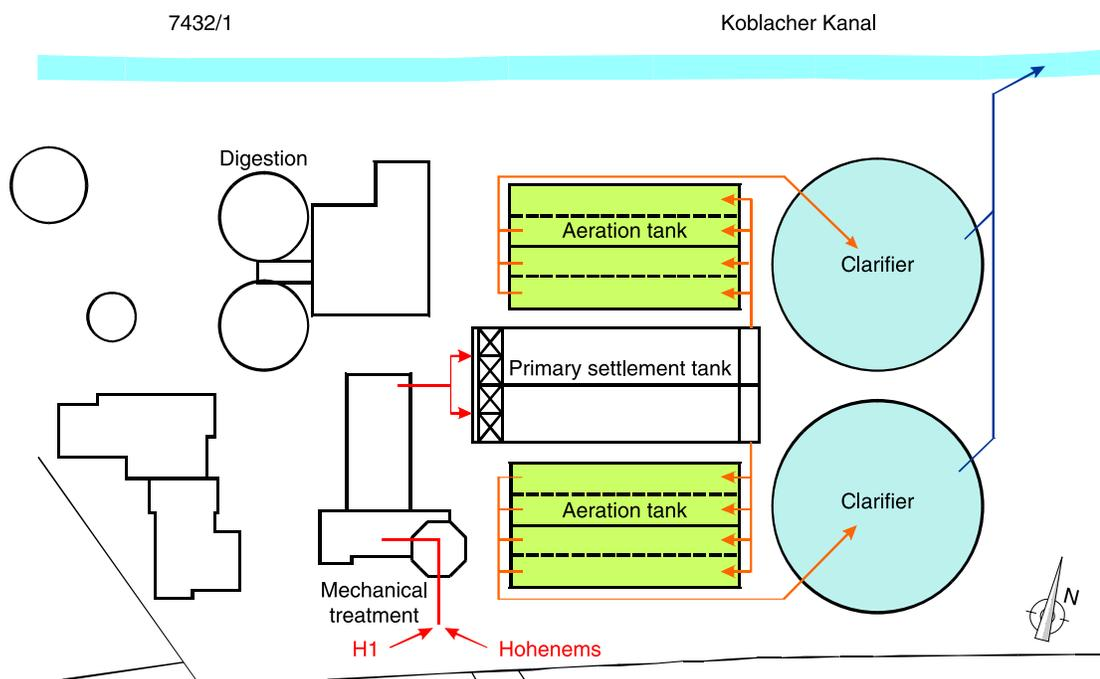
Figure 1 | Initial layout of WWTP Hohenems (1981).
