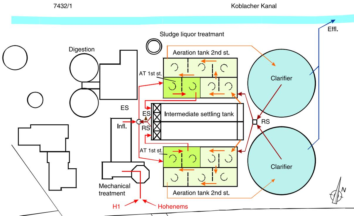
**Figure 2** | New layout of WWTP Hohenems as two stage activated sludge plant according to the HYBRID<sup>®</sup>-process.
