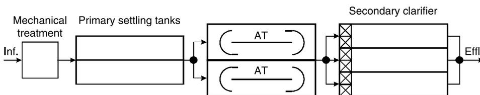
**Figure 3** | Initial layout of WWTP Knittelfeld (1983).
