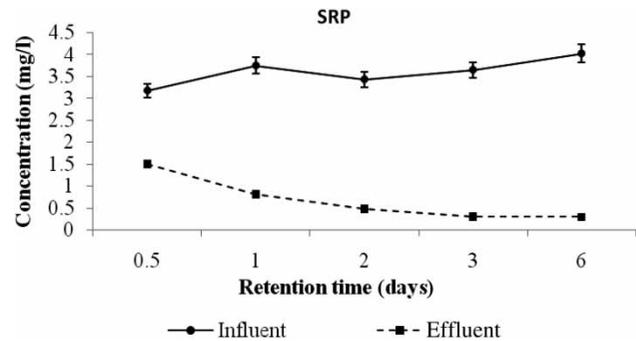
**Figure 7** | SRP concentration in influent and effluent of the system at different retention times.
