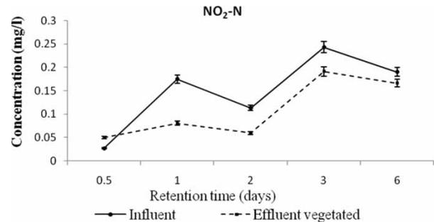
**Figure 4** | NO<sub>2</sub>-N concentration for the influent and effluent from the system at different retention times.
