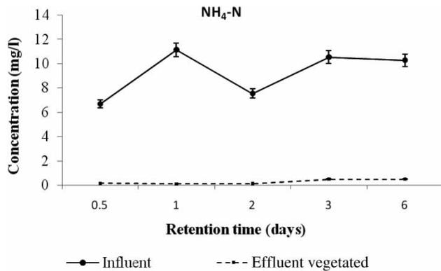
**Figure 5** | Concentration of NH<sub>4</sub>-N for the influent and effluent from the system at different retention times.
