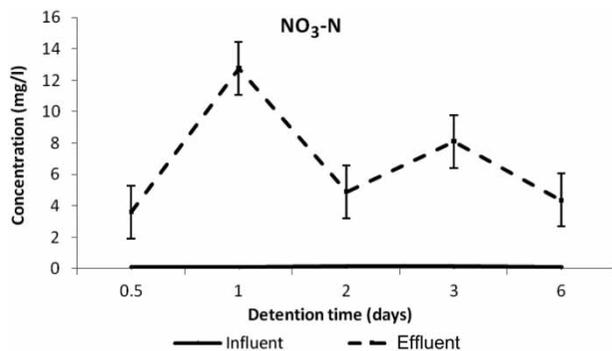
**Figure 3** | Concentration of NO<sub>3</sub>-N at different retention times (vertical bars: standard error).
