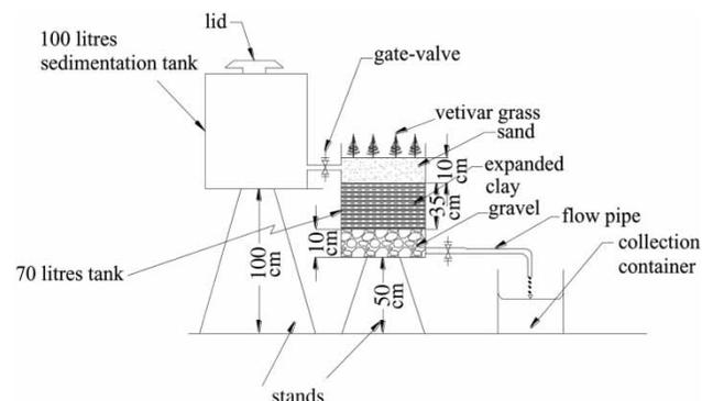
**Figure 2** | The pilot vertical flow constructed wetlands system set-up (units of measurements in centimeters, cm).
