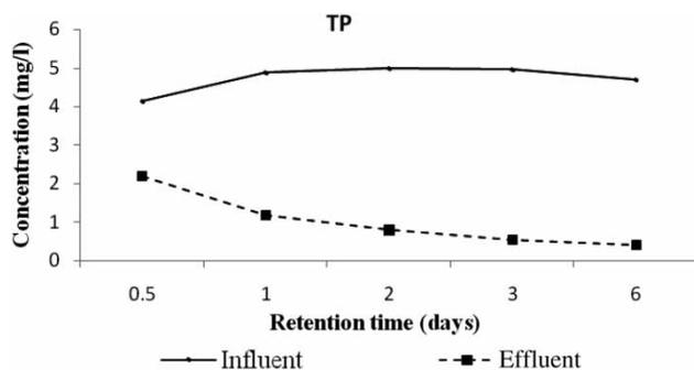
**Figure 6** | Concentration of TP for the influent and effluent from the system at different retention times.
