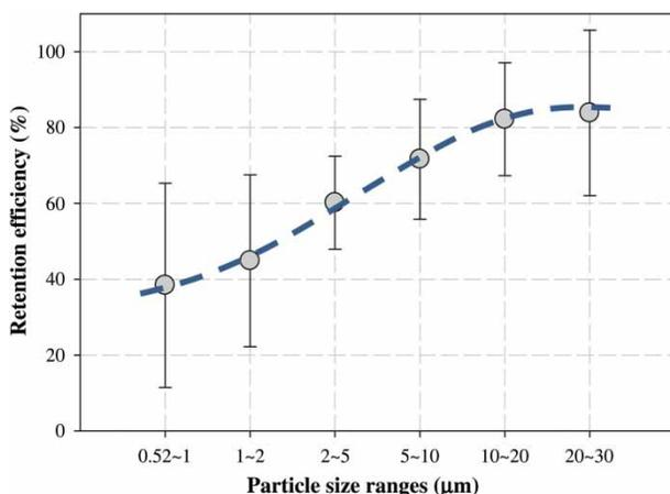
Figure 3 | Particles retention efficiency in sedimentation tank by number.
