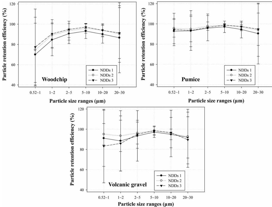
Figure 5 | Effects of recirculation on particle retention efficiency by number.
