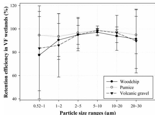
Figure 4 | Particle trapping efficiency in VF wetlands by number.
