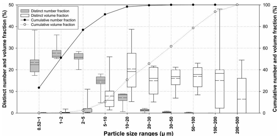
Figure 2 | Particle size distributions in stormwater.
