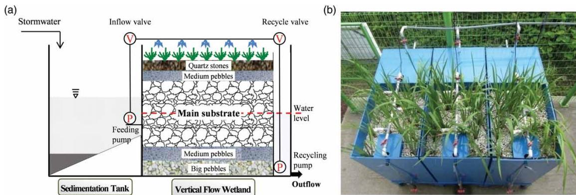
Figure 1 | Schematic diagram (a) and photograph (b) of the compacted wetland systems.
