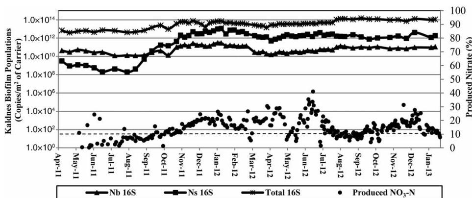
**Figure 4** | Kaldnes biofilm Nb 16S, Ns16S, total 16S population (copies/m<sup>2</sup> of carrier) and percentage of produced nitrate. The dashed lines shows 11% theoretical percent nitrate produced (*Nitrobacter* spp., *Nitrospira* and total bacterial abundance were quantified targeting *amoA*, AMX, and total 16S genes).
