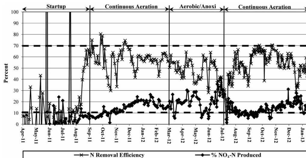
**Figure 1** | Total nitrogen removal (TIN) efficiency and percent nitrate produced in the MBBR pilot. The dashed lines show the 70% objective TIN removal and 11% theoretical value of nitrate produced.
