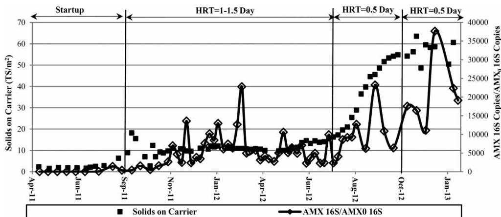
Figure 2 | The ratio of AMX 16S copies for each sample to initial AMX 16S copies and total solids on the carriers.
