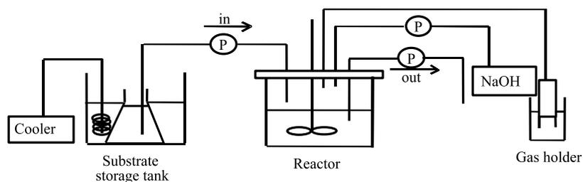
**Figure 3** Experimental apparatus for continuous hydrogen production from okara
