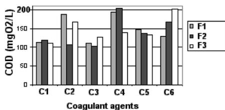
**Figure 1** Removal of COD by C-F
