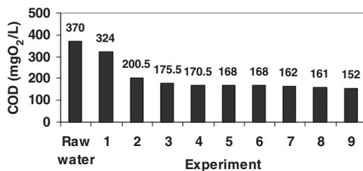
**Figure 6** COD in wastewater treated by the Fenton's method at different reagents doses
