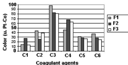
**Figure 2** Removal of color by C-F
