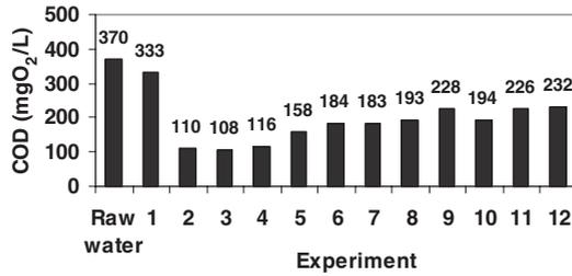
**Figure 5** COD in wastewater treated by the Fenton's method at different weight reagents ratio
