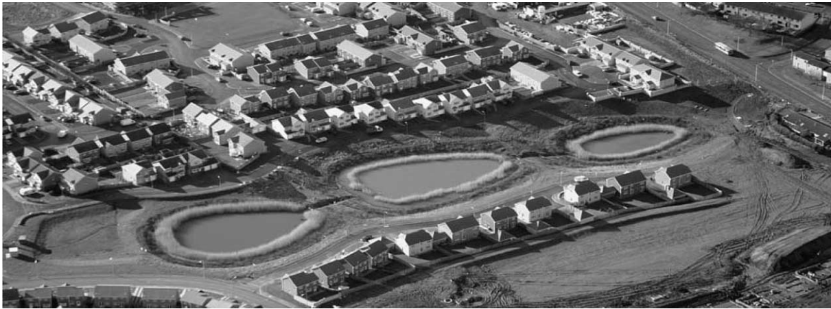
Figure 2 | Cascades pond treatment train, detention basin on the left, at the head of the pond.
