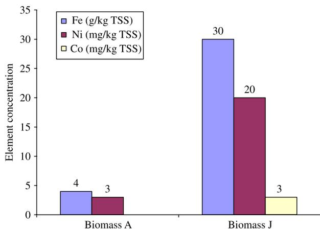
**Figure 4** | Comparison of iron, nickel and cobalt concentration in biomass A (mono digestion of energy crops only) and biomass J (digestion of municipal sludge).
