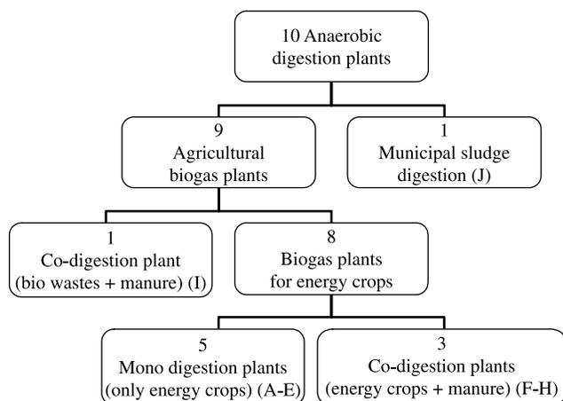
**Figure 1** | Investigated anaerobic digestion plants.
