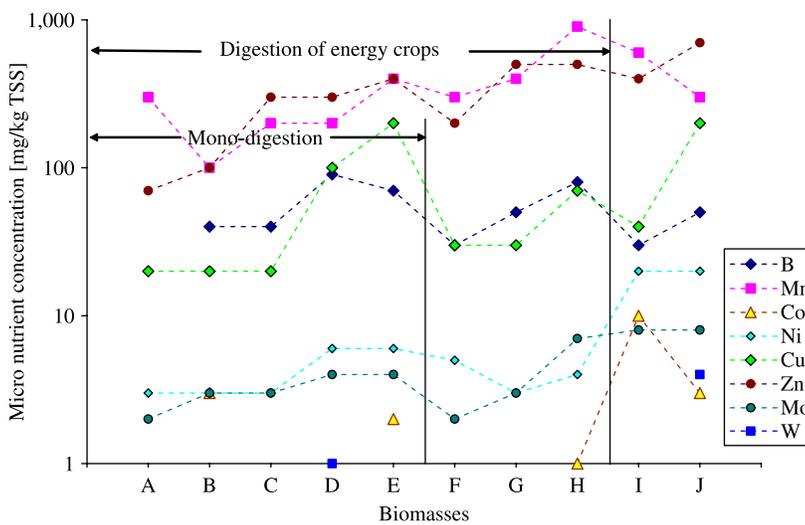
**Figure 3** | Micro nutrients concentration in different biomass [mg/kg TSS].
