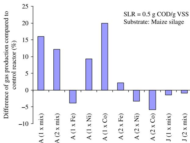
**Figure 5** | Difference in gas production of batch tests with element dosage in comparison to control reactor (only substrate respiration) after 32 d. SLR = 0.5 g COD/g VSS Substrate: Maize silage
