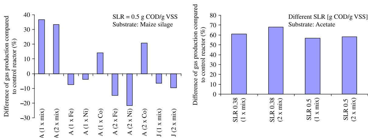
**Figure 7** | Difference in gas production of batch tests with element dosage in comparison to control reactor (only substrate respiration) at day 12 after second addition for maize silage and acetate.
