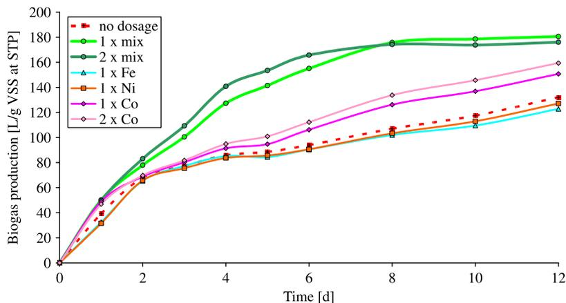
**Figure 6** | Gas production in different anaerobic batch tests with maize silage at SLR = 0.5 g COD/g VSS.
