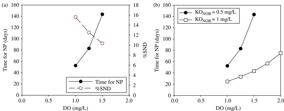
**Figure 3** | Summary of the results applying the low DO setpoint strategy: (a) Time for NP and %SND at different DO setpoints; (b) Impact of  $K_{O\_NOB}$  on the achievement of the nitrite pathway.
