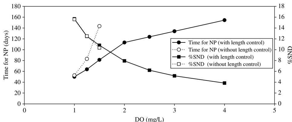
**Figure 5** | Comparison of the Time for NP and %SND as functions of DO setpoint, with and without aeration phase length control.
