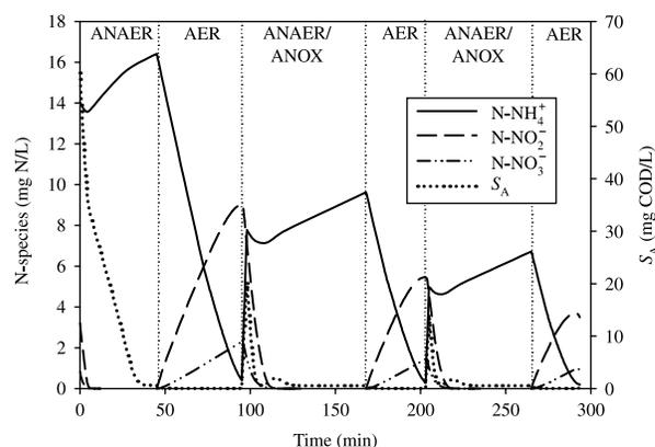
Figure 1 | Ammonium, nitrite, nitrate and RBCOD ( $S_A$ ) profiles in a typical SBR cycle.
