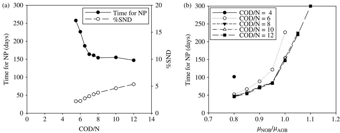
**Figure 2** | Summary of the results applying the control of the aerobic phase length strategy: (a) at different COD/N values for  $\mu_{NOB\_MAX} = \mu_{AOB\_MAX} = 1 \text{ d}^{-1}$ , (b) at different COD/N and  $\mu_{NOB\_MAX}/\mu_{AOB\_MAX}$  ratios.
