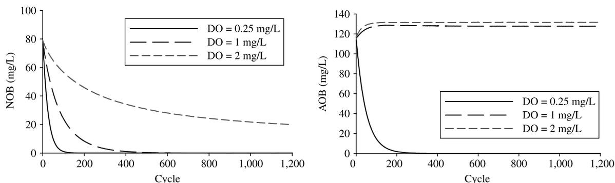
**Figure 4** | Evolution of AOB and NOB at different DO values ( $K_{O_{AOB}} = K_{O_{NOB}} = 0.5 \text{ mg/L}$ ).
