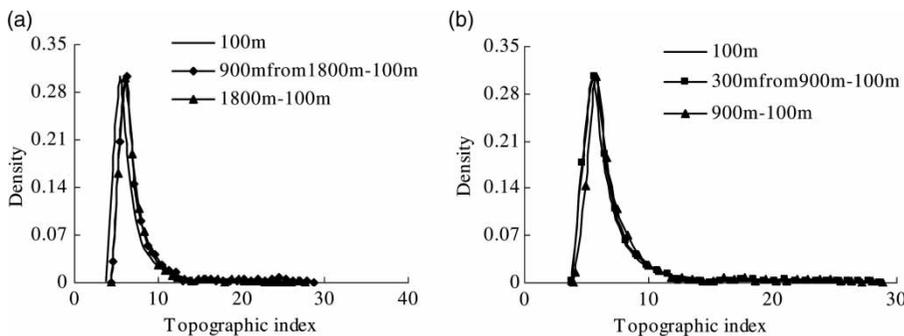
**Figure 6** | Frequency curve of fractal slope with and without downscaling. (The meaning of '100 m', '900 m' and '300 from 900-100 m' are as in Figure 4. '900 m from 1,800-100 m' means the fractal slope at the target resolution of 100 m computed from the 900 m DEM which is downsampled from 1,800 m DEM.)
