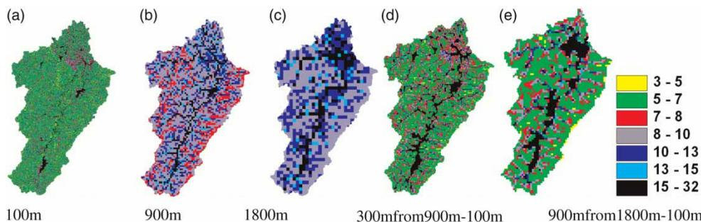
**Figure 7** | Spatial distribution of topographic index and scaled topographic index at different DEM resolutions. (The meaning of '100 m', '900 m' and '300 from 900m-100 m' are as in Figure 4. '900 m from 1,800 m-100 m' means the fractal slope at the target resolution of 100 m computed from the 900 m DEM which is downsampled from 1,800 m DEM.)
