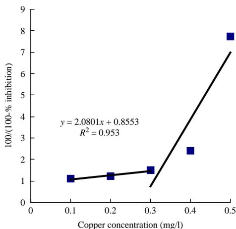
**Figure 5** | Regression of  $100/(100 - \% \text{ inhibition})$  with copper concentrations. The inhibition constant was determined as the inverse of the slope of the regressed line (the first three data points).
