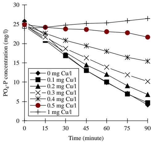
**Figure 3** | Aerobic dynamics of soluble  $\text{PO}_4\text{-P}$  under copper concentrations ranging from 0 mg/l to 1 mg/l.
