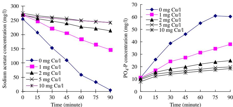
**Figure 1** | Anaerobic dynamics of soluble sodium acetate and PO<sub>4</sub>-P under copper concentrations from 0 mg/l to 10 mg/l.
