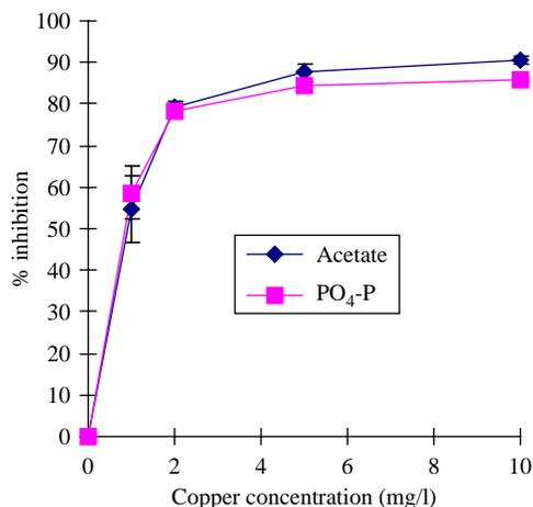
**Figure 2** | Inhibition of microbial activity on anaerobic acetate uptake and phosphorus release under copper concentrations from 0 mg/l to 10 mg/l based on the zero-order regression.
