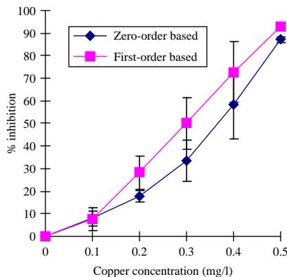
**Figure 4** | Inhibition of microbial activity on aerobic phosphorus uptake under copper concentrations from 0 mg/l to 0.5 mg/l based on both the zero-order and the first-order regressions.
