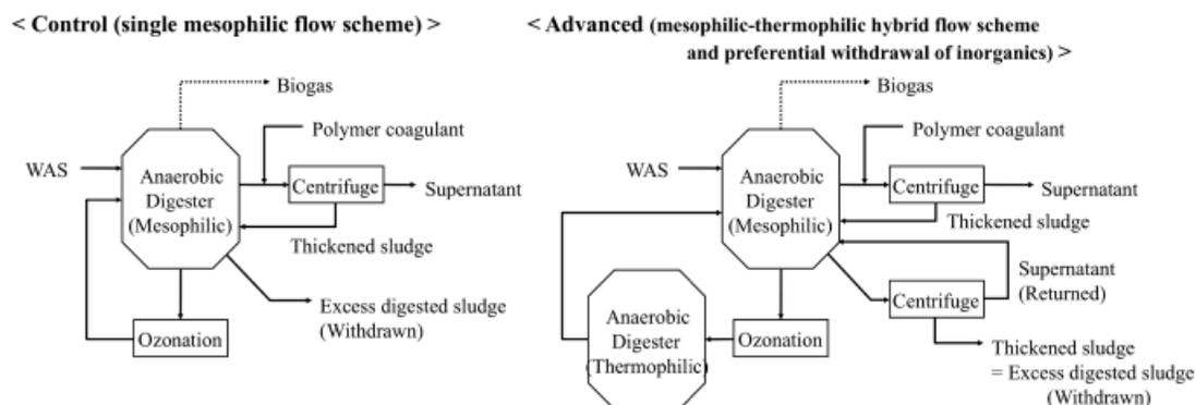
Figure 1 | Experimental process configuration.
