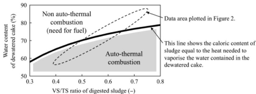
**Figure 3** | Auto-thermal combustion of dewatered sludge cake.
