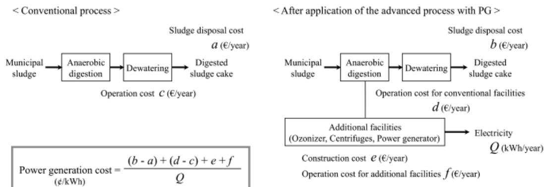
**Figure 4** | Power generation (PG) cost for the advanced anaerobic digestion process.
