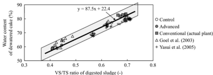
Figure 2 | Relationship between the VS/TS ratio and water content of the dewatered cake.
