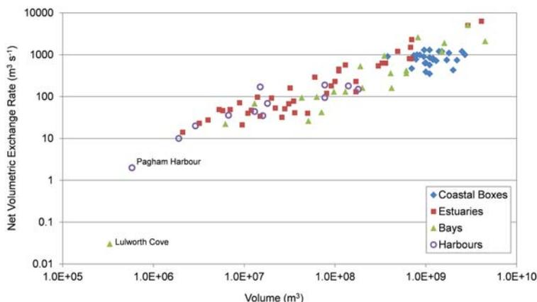
FIG. 5. Net exchange rate vs. volume, based on data in Dewar *et al.* (2011).
