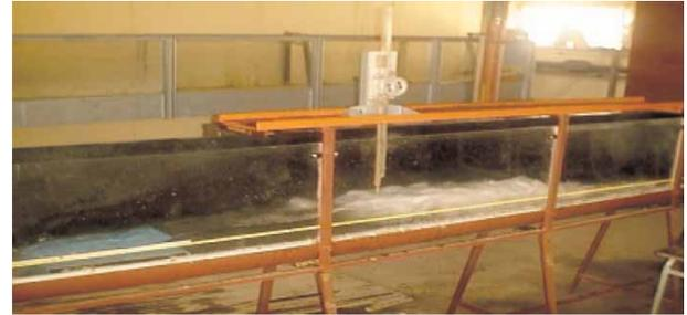
Figure 4 | Hydraulic jump controlled by a broad sill in U-channel.
