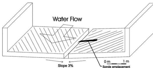
Figure 2 | Multiparametric probe emplacement in the Chorrito Stream.
