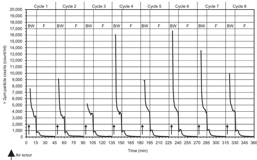
**Figure 2** | The variation of total particle counts (>2  $\mu\text{m}$ ) for 8 successive clean bed backwash (BW) and filter ripening cycles (F).
