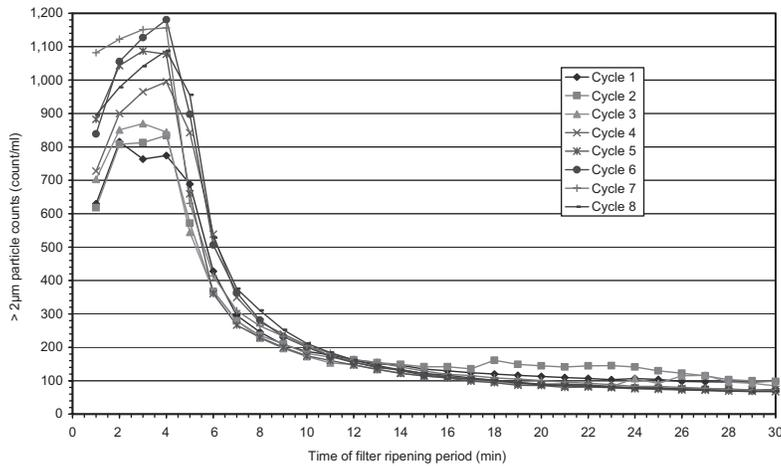
**Figure 5** | The variation of total particle counts (> 2  $\mu\text{m}$ ) during the 8 filtration cycles.
