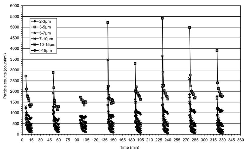
**Figure 3** | The variation of differential particle counts for 8 successive backwash cycles (filtration data omitted).
