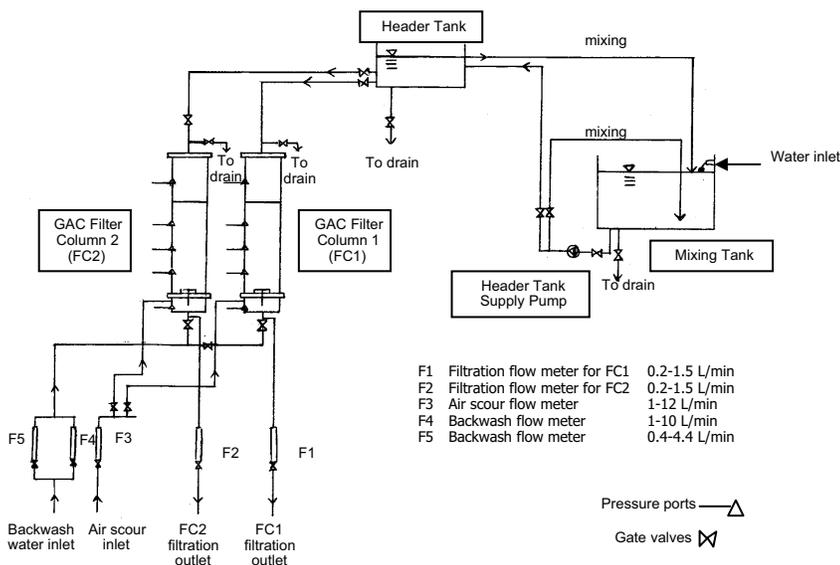
**Figure 1** | Schematic diagram of the filter column apparatus used in the laboratory study.
