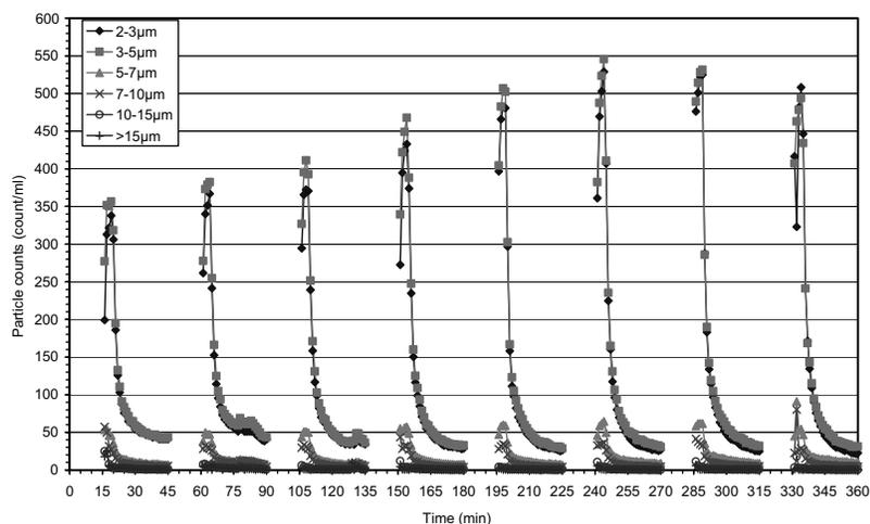
**Figure 4** | The variation of differential particle counts during the filter ripening period after each successive backwash.
