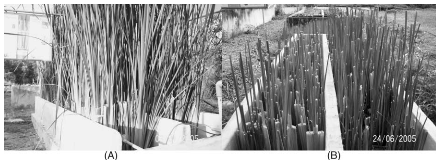
Figure 1 A: Subsurface-flow constructed wetland (SSFCW), B: Harvesting of Typha angustifolia l. plants grown in SSFCW units
