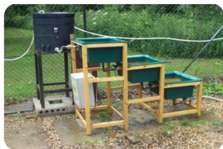
The prototype – cascaded vertical flow CW
