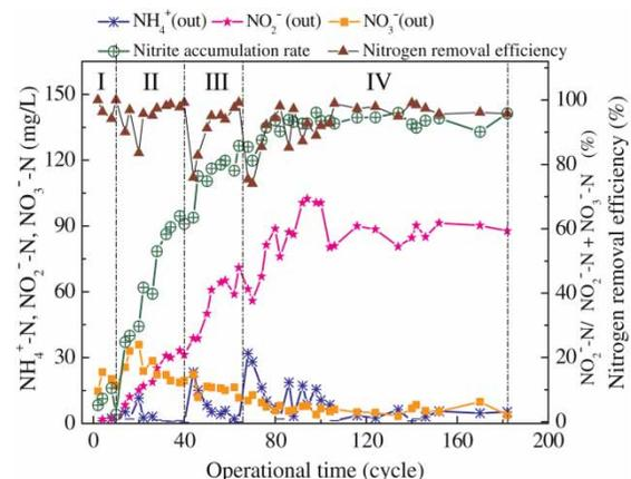
Figure 4 | Nitrification performance during the granulation process.
