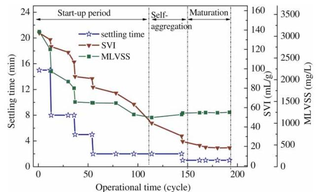
Figure 1 | Variations of settling time, SVI and MLVSS during the granulation.
