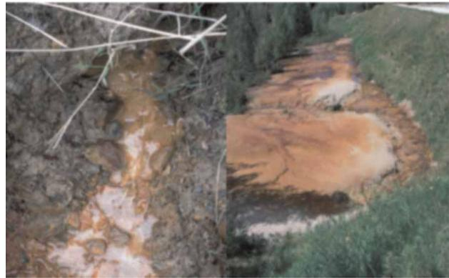
**Figure 3** | Examples of seepage water sampling points at showing the upper seepage area at the toe of the upper section of the dam (Heikkinen 2009).
