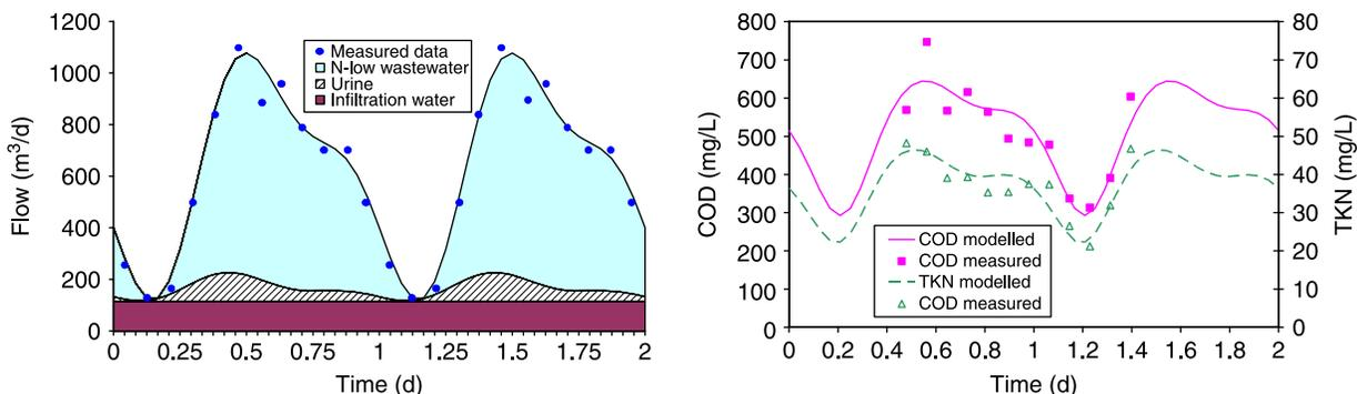
Figure 1 | Comparison of measured and modelled flow (left) and concentrations of COD and TKN (right).
