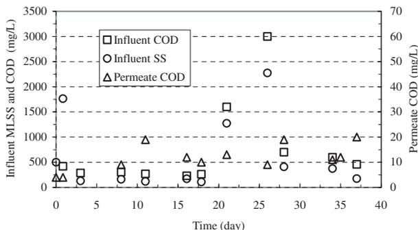
**Figure 4** Variation of permeate COD for the air-lift module in accordance with the fluctuation of influent COD and MLSS
