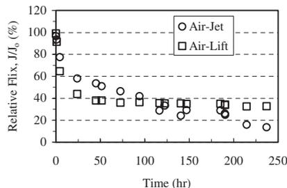
**Figure 6** Comparison of flux decline between air-jet and air-lift module
