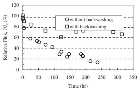
**Figure 5** Effect of backwashing on flux performance for the air-jet module
