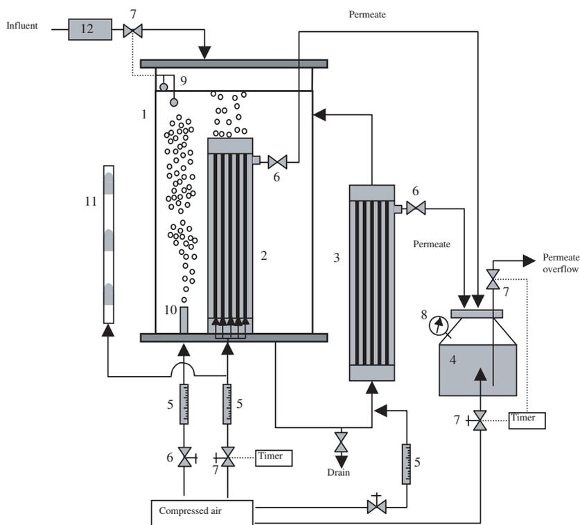
**Figure 1** Schematic diagram of the experimental set-up for the submerged MBR; (1) bioreactor, (2) air jet module, (3) air lift module, (4) pressurised backwashing tank, (5) flow meter, (6) adjustment valve, (7) solenoid valve, (8) pressure gauge, (9) level sensor, (10) diffuser, (11) visualization tube, (12) prefilter
