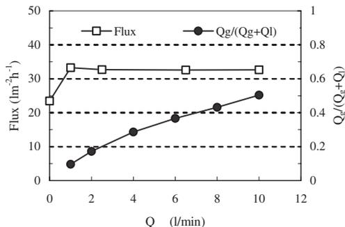
**Figure 2** Flux decline as a function of air flow-rate for the air-lift module during filtration of mixed liquor of activated sludge
