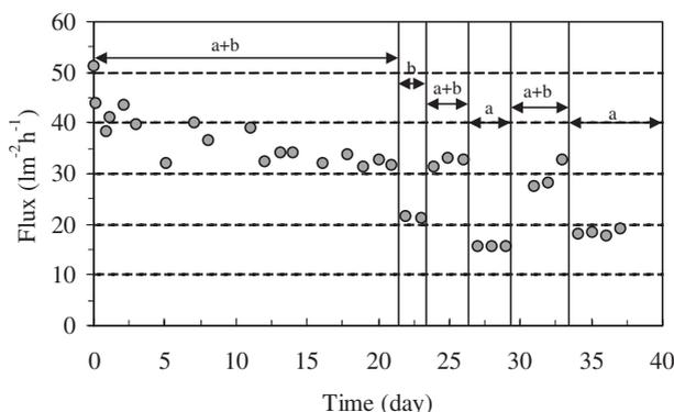
**Figure 3** Effect of backwashing and air-injection on flux performance of the air-lift module; (a) air only, (b) backwashing only, (a+b) air and backwashing together
