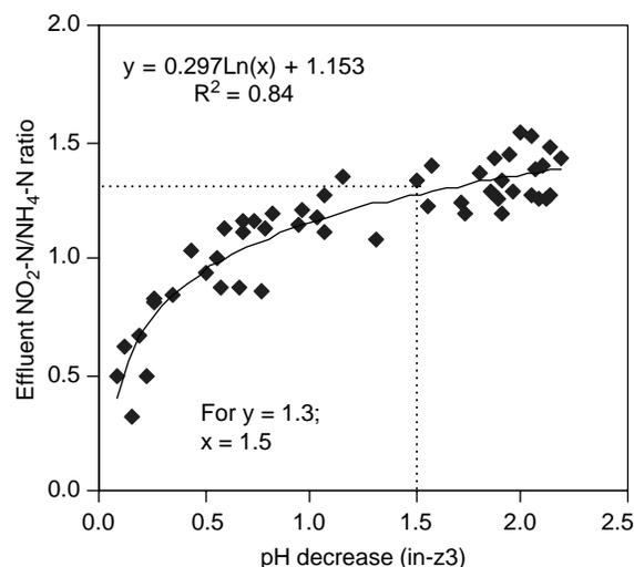
**Figure 3** The pH decrease and the effluent  $\text{NO}_2\text{-N}/\text{NH}_4\text{-N}$  ratio in R1 (based on data from 2003 and 2004)
