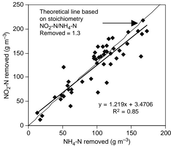
**Figure 9** Removal of ammonium and nitrite nitrogen in R2
