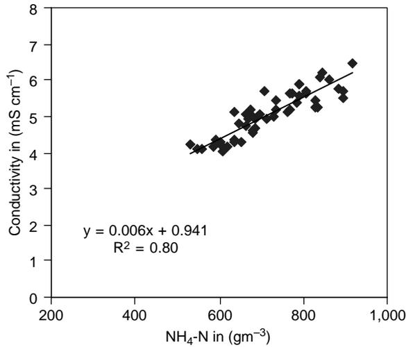
**Figure 5**  $\text{NH}_4\text{-N}$  concentration and conductivity in the influent to the pilot plant
