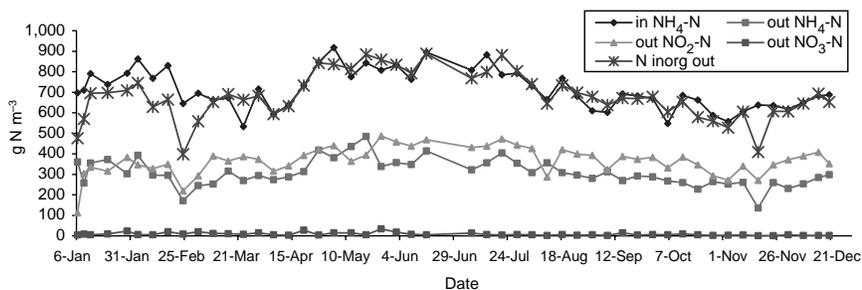
**Figure 2** Variations of inorganic nitrogen forms in the partial nitrification reactor (R1)
