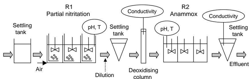
**Figure 1** Scheme of the semi-industrial scale pilot plant at Himmerfjärden WWTP
