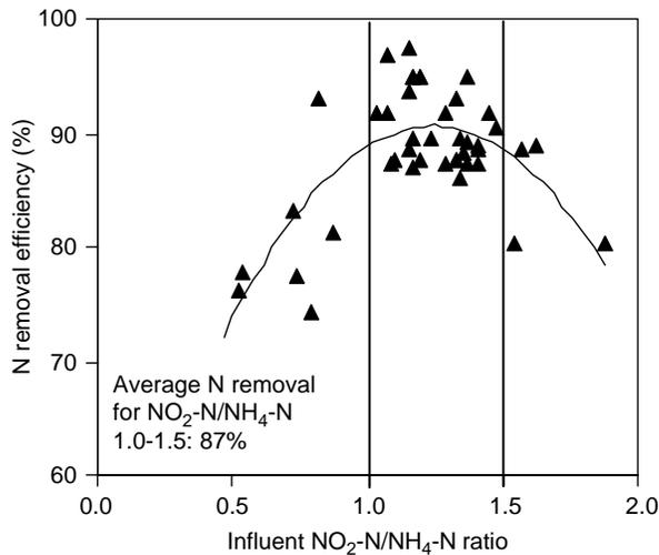
**Figure 10** The influent  $\text{NO}_2\text{-N}/\text{NH}_4\text{-N}$  ratio and the nitrogen removal efficiency in R2
