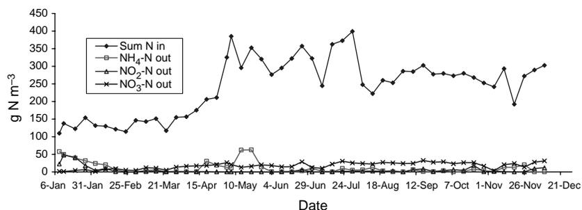
**Figure 7** Inorganic nitrogen forms concentration in the influent and effluent (R2)
