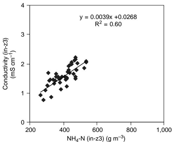
**Figure 6** Removed ammonium and removed conductivity in R1
