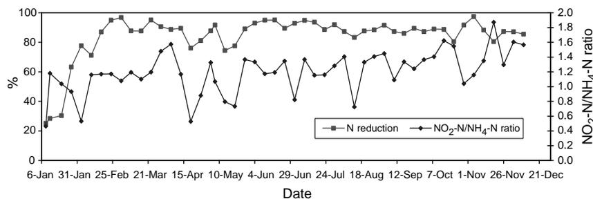
**Figure 8**  $\text{NO}_2\text{-N}/\text{NH}_4\text{-N}$  ratio in the influent and total inorganic nitrogen removal efficiency (R2)
