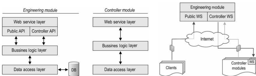
**Figure 2** | Design of the AqS architecture: (left) the engineering module; (middle) the controller module; (right) WS communication between software components.
