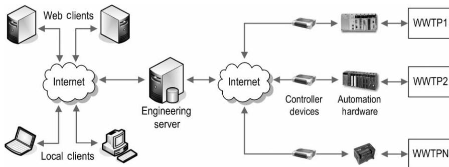
Figure 3 | Hardware architecture of AqS.
