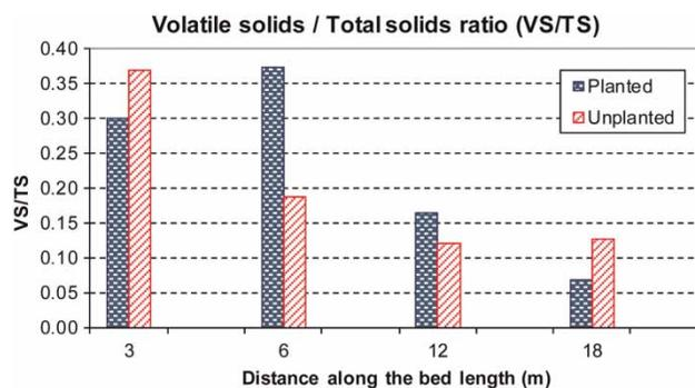
**Figure 3** | Ratio of volatile to total solids (VS/TS) in the filter medium along the planted and unplanted units.
