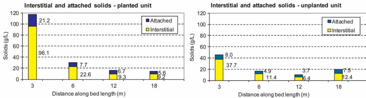
Figure 4 | Proportion of interstitial and attached solids along the beds of the planted and unplanted units.
