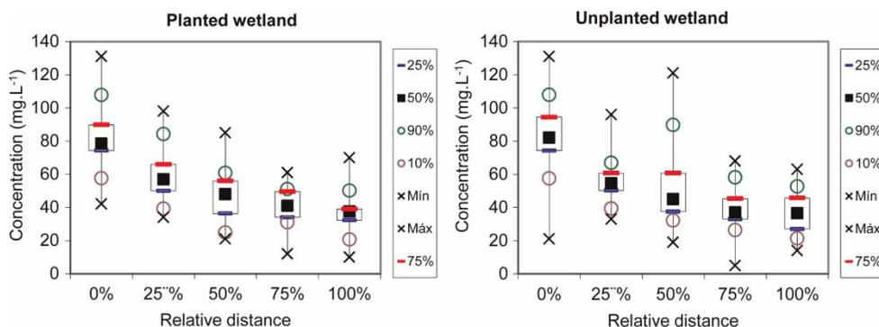
**Figure 2** | Box-plot for the decay of the concentration of organic matter (filtered COD) along the wetlands.
