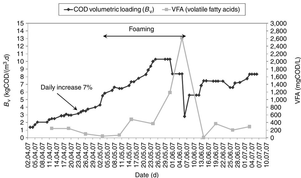
**Figure 3** |  $B_v$  increase and VFA concentrations in the single-stage lab-scale methane reactor seeded with digested sludge from Budapest's WWTP and fed with silaged SBP.
