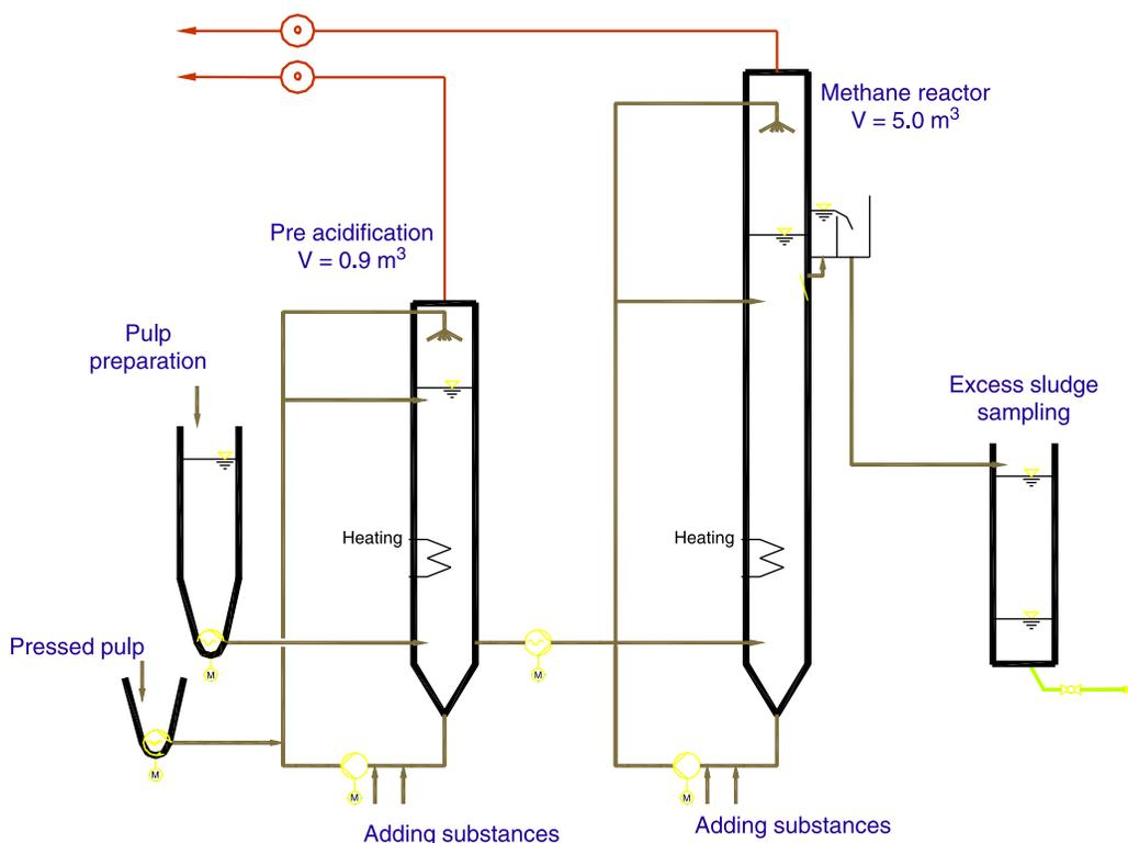
Figure 1 | Pilot plant No. 1, two-stage digestion process with pre-acidification.
