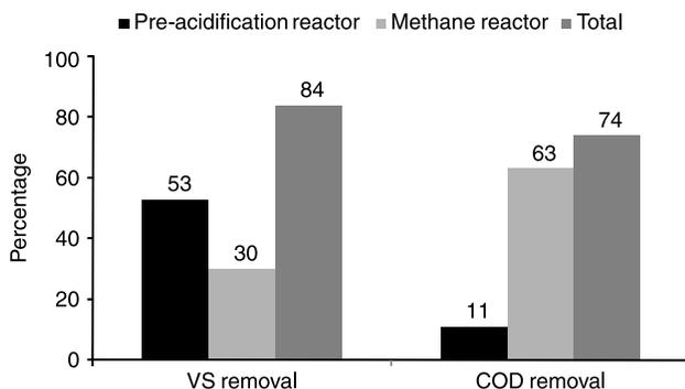
**Figure 2** | Removal efficiency of VS and COD in the two-stage configuration.
