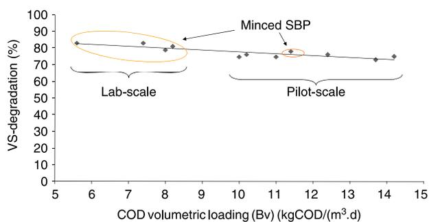
**Figure 4** | TS degradation in correlation to COD volumetric load (Bv), single-stage configuration.
