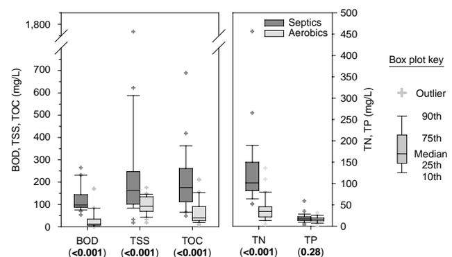
**Figure 3** | Comparison of aerobic system and septic tank effluent quality showing 10th, 25th, 50th (median), 75th and 90th percentiles (numbers in brackets indicate  $P$ -value, values in bold indicates statistically significant result).
