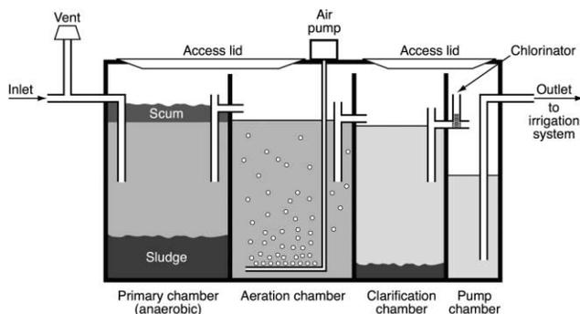
**Figure 1** | Cross-section of a typical aerobic wastewater treatment system, showing separate chambers for primary (anaerobic) treatment, aeration and clarification, and chlorine tablets in the chlorinator prior to the pump chamber.
