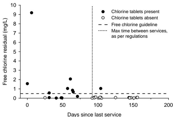
**Figure 4** | The relationship between the free chlorine residual and time since last service.
