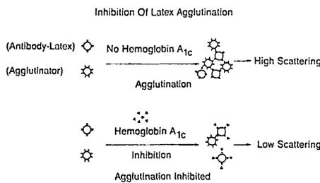
**Figure 1**—Assay principle used in determination of HbA<sub>1c</sub> concentrations. Slope of inhibitor and latex agglutination curve is sigmoidal. A 4-parameter curve fit is used to plot response vs. concentration for calculations of unknowns.
