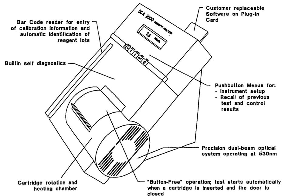
**Figure 3**—DCA 2000 chemistry analyzer.
