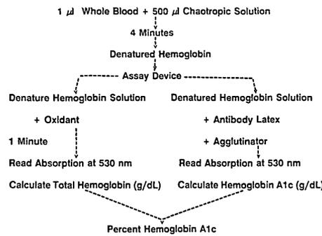
**Figure 2**—Chemical reactions occurring within reagent cartridge. Ratio of HbA<sub>1c</sub> to total Hb is calculated to determine percentage HbA<sub>1c</sub>.
