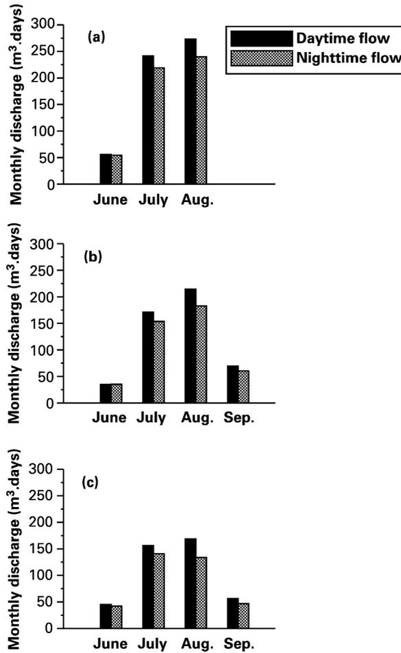
**Figure 2** Monthly distribution of daytime (0900–2100 hours) and night-time (2100–0800 hours) mean discharge observed near the snout of Dokriani Glacier during three ablation seasons (a) 1996, (b) 1997 and (c) 1998
