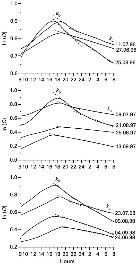
**Figure 6** Variation in recession trends of discharge on clear weather days during three ablation seasons (1996–1998).  $k_b$  and  $k_c$  represent the runoff delaying response of the ablation and accumulation zones, respectively
