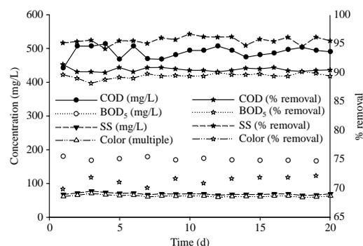
**Figure 2** | Variations of COD, BOD<sub>5</sub>, SS, color by coal cinder filtration. Experimental conditions: Influent wastewater: COD, BOD<sub>5</sub>, SS and color were 4,200–4,500 mg/L, 600–630 mg/L, 650–680 mg/L and 600–620 (multiple); temperature: room temperature; Hydraulic retention time: 1–1.5 h.
