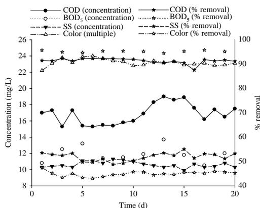
**Figure 4** | Variations of COD, BOD<sub>5</sub>, SS, color in biological contact oxidation tank. Experimental conditions: Influent wastewater: COD, BOD<sub>5</sub>, SS and color were 180–210 mg/L, 130–140 mg/L, 20–23 mg/L and 40–44 (multiple); temperature: room temperature; Hydraulic retention time: 2.7 h.
