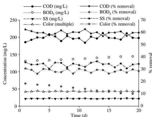
**Figure 3** | Variations of COD, BOD<sub>5</sub>, SS, color in hydrolysis-acidification tank. Experimental conditions: Influent wastewater: COD, BOD<sub>5</sub>, SS and color were 420–440 mg/L, 160–180 mg/L, 60–70 mg/L and 60–70 (multiple); temperature: room temperature; Hydraulic retention time: 8 h.
