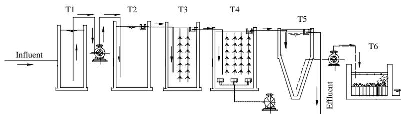
**Figure 1** | Schematic diagram of experimental set-up. T1: collecting well; T2: grit chamber; T3: hydrolysis-acidification tank; T4: biological contact oxidation tank; T5: Secondary sedimentation tank; T6: sludge drying bed.
