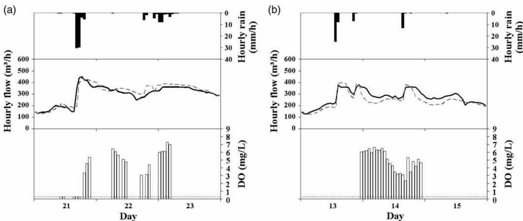
**Figure 4** | Hourly flow, rain and DO concentration at the outlet of the sanitary sewer system of Coronel Oviedo during (a) Rain-event 1 and (b) Rain-event 2 (the dashed line represents the modelled flow; the dotted line represents the dry weather DO concentration).
