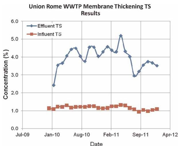
Figure 6 | Union Rome WWTP thickening results of aerobic digestion system.
