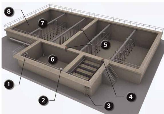
**Figure 1** | General membrane thickening aerobic digestion process.
