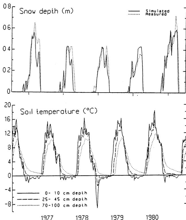
Fig. 6. Simulated and measured snow depth and simulated soil temperatures.
