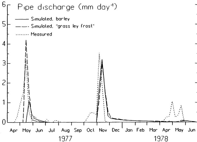
Fig. 11. Simulated and measured weekly mean values of pipe discharge during a selected period. Simulated values represent barley (the same as in Fig. 10) and one additional simulation with frost depths according to grass ley but with hydrological properties according to barley.
