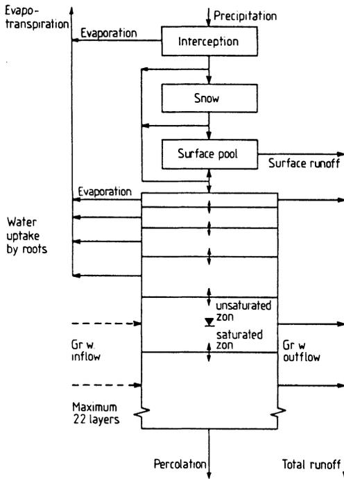
**Fig. 2.** Model structure of the water and heat model. All flows in the soil profile except water uptake by roots represent both water and heat (modified from Jansson and Halldin 1979).
