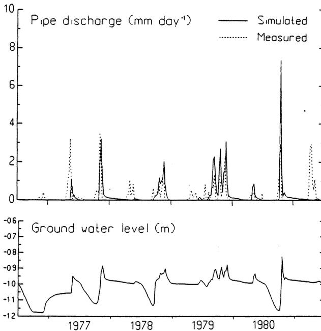
Fig. 10. Simulated and measured weekly mean values of pipe discharge and simulated ground water levels. Simulated values represent barley.
