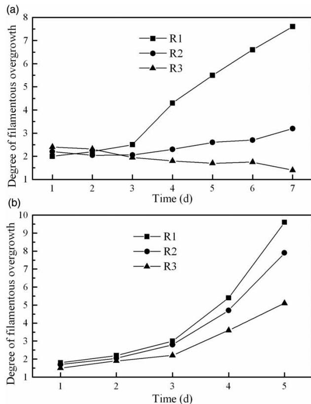
Figure 4 | Variation of the degree of filamentous overgrowth  $\Delta$  during the study of (a) carbon source type, (b) temperature.
