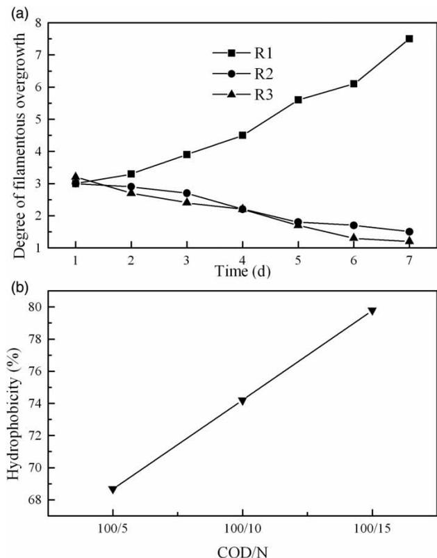
**Figure 5** | (a) Variation of the degree of filamentous overgrowth  $\Delta$  and (b) cell hydrophobicity in reactors during the experiment of COD/N ratio.
