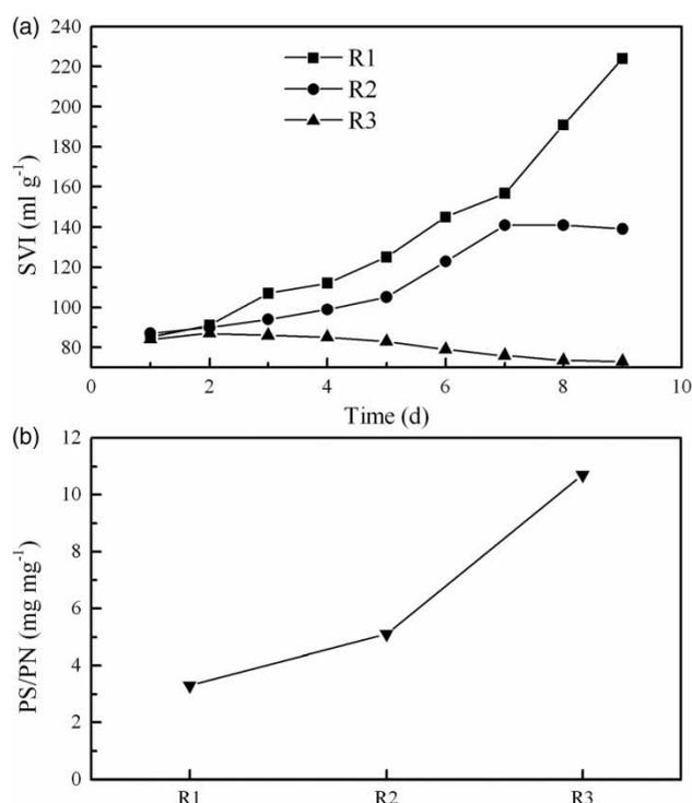
Figure 2 | Evolution of (a) SVI profiles and (b) ratio of PS to PN in reactors during the study of DO.
