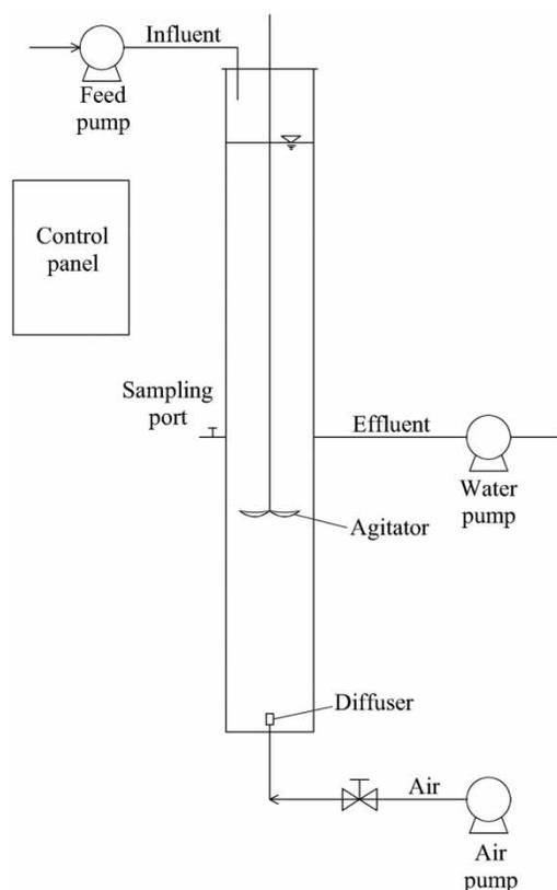
Figure 1 | Schematic diagram of aerobic granular sludge SBR.
