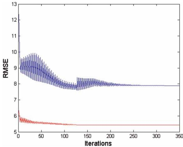
**Figure 6** | ANFIS train based on two sets of data; upper: check dataset and lower: train dataset.
