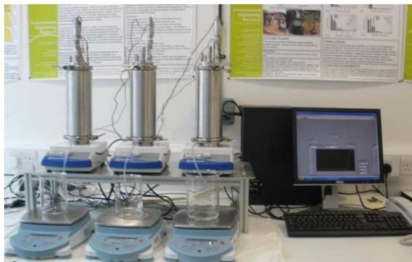
**Figure 1** | Stirred cells filtration system.
