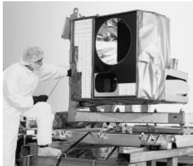
FIG. 2. MODIS Protoflight Model (first MODIS flight unit for EOS AM-1). Radiative cooler faces camera with scan mirror on the lower right.
