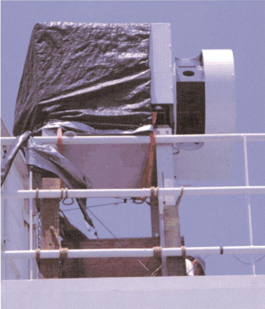
FIG. 5. The M-AERI installed on the NOAA S *Ronald H. Brown*. The instrument is on the forward 02 deck at the starboard railing. The field of view intersects the sea surface ahead of the bow wave.
