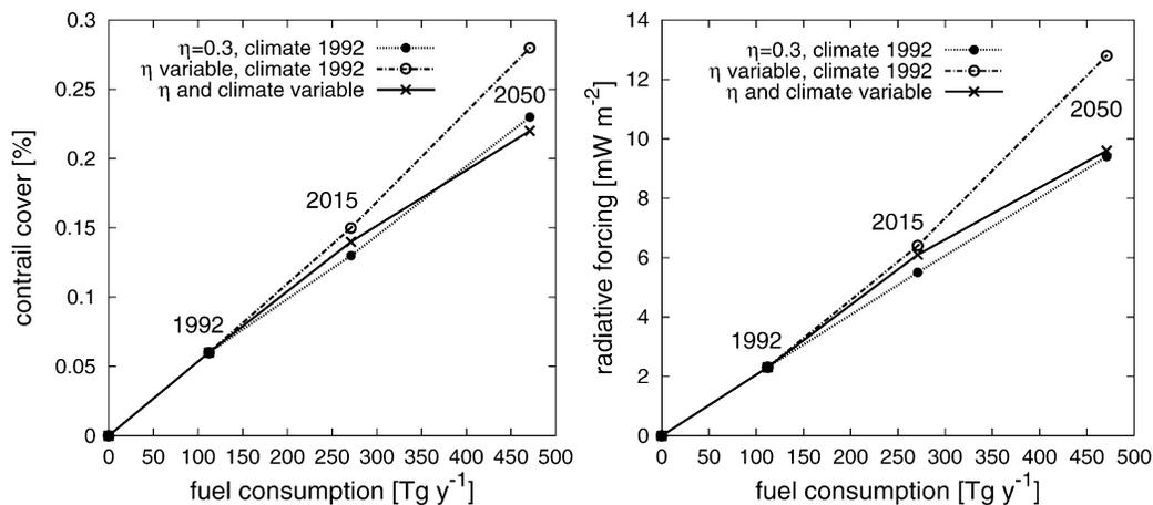
FIG. 8. (left) Annually and globally averaged total contrail cover and (right) net radiative forcing in 1992, 2015, and 2050, displayed as a function of global annual fuel consumption. Changes in air traffic, propulsion efficiency ( $\eta$ ), and climate are taken into account.
