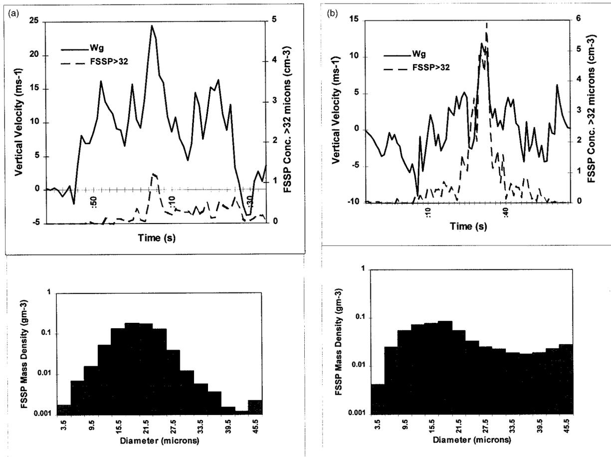
FIG. 1. FSSP droplet concentrations greater than  $32 \mu\text{m}$  and vertical velocities measured on two passes through a cloud seeded with hygroscopic flares on 9 October 1990. The histograms show the distribution of cloud water ( $\text{gm}^{-3}$ ) between 2 and  $47 \mu\text{m}$  averaged over 1 km centered around the maximum updraft speeds: (a) 2 min after seeding commenced at cloud base and (b) 6 min after seeding commenced (see text for further details).
