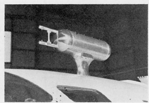
FIG. 1. Optical-array particle size spectrometer installed on NCAR Sabreliner.
