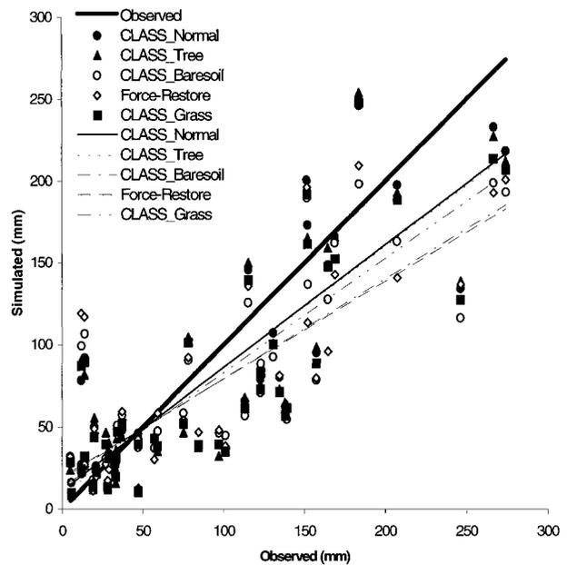
FIG. 6. Scatterplot of 48-h accumulated precipitation (in mm) for five 10-km runs (MC2/CLASS with actual vegetation conditions, uniform coniferous trees, grass, and bare soil, and MC2/force-restore) vs observations from the 46 rain gauges. Regression lines from a least squares fit are also provided.
