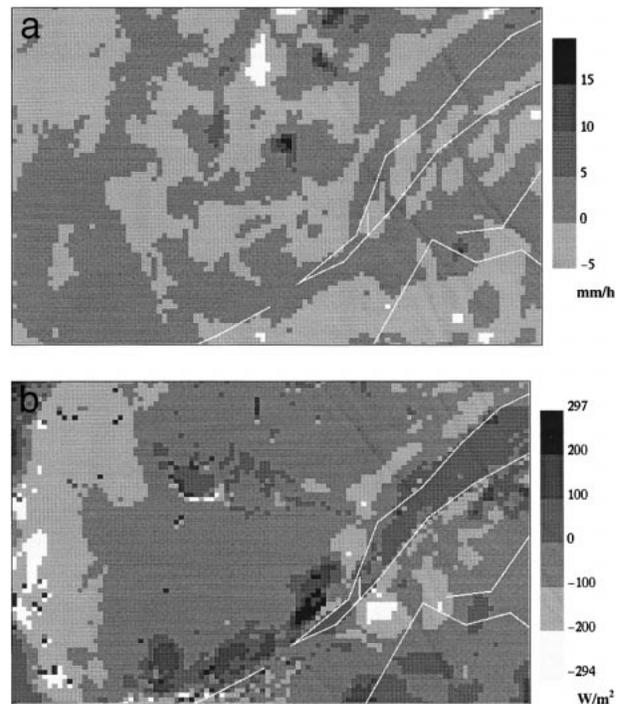
FIG. 8. (a) The differences in precipitation rate of MC2/CLASS and MC2/force–restore at 5 km taken at 1800 UTC 20 Jul 1996. (b) The differences in sensible heat flux of MC2/CLASS and MC2/force–restore at 5 km taken at 1800 UTC 20 Jul 1996.
