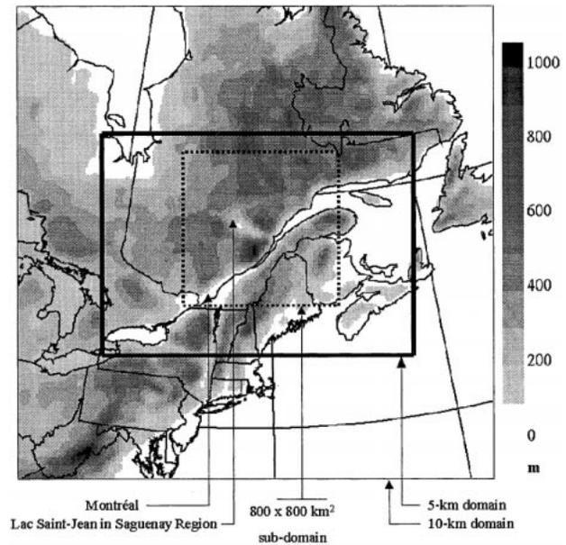
FIG. 1. Simulation domains for the two resolutions: 1)  $331 \times 231$  grid points at 5 km, and 2)  $251 \times 251$  grid points at 10 km. Both domains are centered at  $48^\circ\text{N}$  and  $71^\circ\text{W}$ . The dotted line shows the subdomain covering the Saguenay region and its immediate vicinity discussed in subsequent figures. The grayscale shows surface topography (m) at 10-km resolution.
