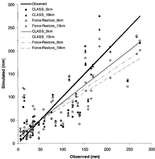
FIG. 5. Scatterplot of 48-h accumulated precipitation (in mm) from MC2/CLASS and MC/force-restore at 10- and 5-km resolutions vs observations from 46 rain gauges. Regression lines from a least squares fit are also provided.
