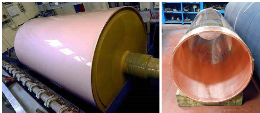
FIG. 1. Electroformed copper chill roll during manufacture (left) and copper shell produced by electroforming (right), with typical dimensions of 1 m diameter, 2.5 m long and 16 mm wall thickness.
