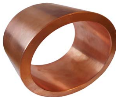
FIG. 4. Copper shell (10 cm inner diameter, 20 cm long, 1 cm thick) electroformed on the 100 L tank.
