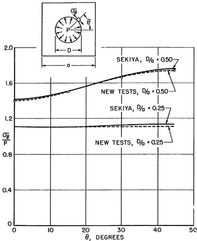
Fig. 5 Hydrostatically loaded central circular hole in a square plate. (Comparison of results obtained theoretically by Sekiya and results obtained from a new series of photoelastic tests.)
