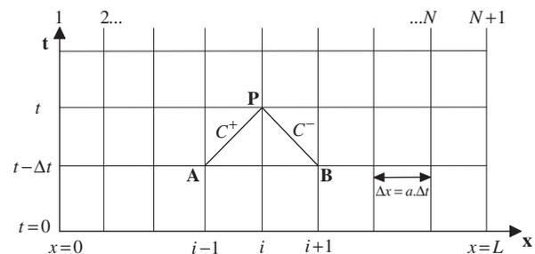
Figure 1 | Characteristic grid with specified time intervals.
