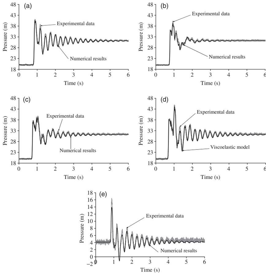
**Figure 7** | Numerical results of the viscoelastic transient solver versus transient pressure data for the leak test ( $Q_0 = 2.47$  L/s;  $Q_L = 0.73$  L/s) at different locations (distance from the pump section): (a) P06 (7.20 m), (b) P02 (32.40 m), (c) P01 (46.10 m), (d) P07 (67.00 m) and (e) P05 (-0.20 m).
