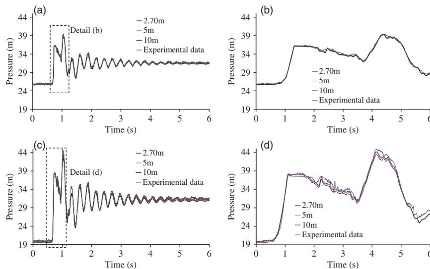
**Figure 11** | Calculated pressure heads for optimal leak location versus experimental data for: (a) Case A, (b) detail of first pressure peak for Case A, (c) Case B and (d) detail of first pressure peak for Case B.
