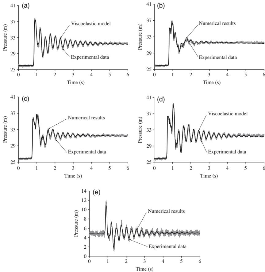
**Figure 6** | Numerical results of the viscoelastic transient solver versus transient pressure data for the leak test ( $Q_0 = 1.84$  L/s;  $Q_L = 0.84$  L/s) at different locations (distance from the pump section): (a) P06 (7.20 m), (b) P02 (32.40 m), (c) P01 (46.10 m), (d) P07 (67.00 m) and (e) P05 (-0.20 m).
